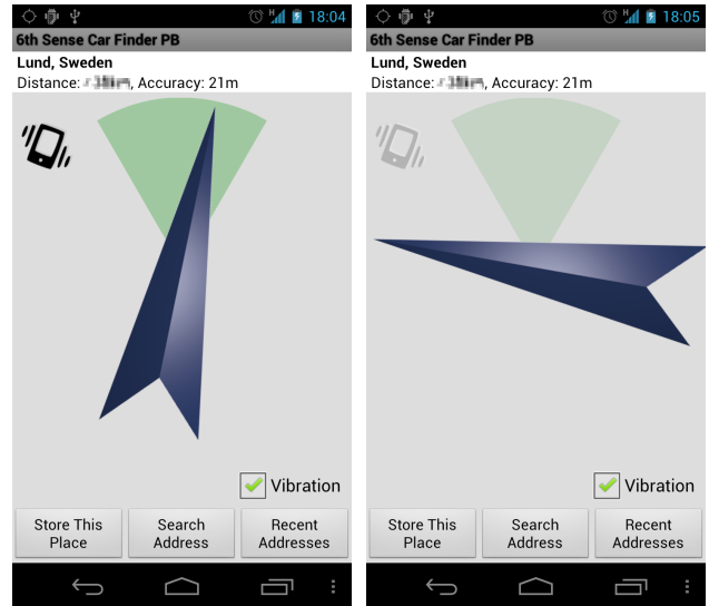
Figure 3. Main view of the Car Finder App: visual cues help the user to quickly grasp how the vibration feedback works.
