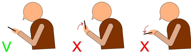
Figure 4. The tilt of the device is used to determine whether the user is likely to be checking the display.
