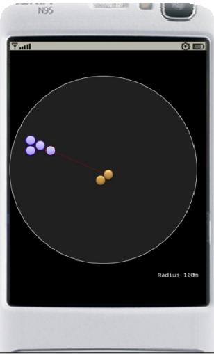
**Figure 2.** Screenshot of the visual component of FriendSense: direction and distance of all friends are shown in a radar-like UI. In the illustrated situation, two friends have strayed away from the group, which is to the left-hand side. The red dashed line indicates which friend the user has selected to be displayed via the tactile feedback.
