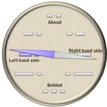
**Figure 3.** The vibro-tactile friend sense: the grey bars visualize the vibration pattern that would be played to indicate the respective directions. In this picture, the violet pattern (long-short) is played indicating that the friend is to the left-hand side.
