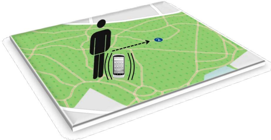
Fig. 1. A "tactile compass" encodes in which direction and how far a place is located from the perspective of the user by vibration patterns generated with a common mobile phone. Unlike wide-spread turn-by-turn wayfinding systems, this tactile compass allows a more traditional sense of navigation, empowering people to revive their inherent navigation skills.
